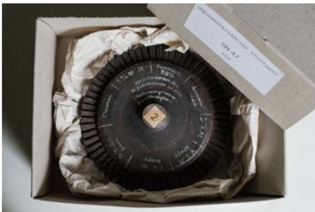
Holzwarth used test wheels like this one to test the materials for the gas turbine blades. Not all material samples withstood the fire gases of 600 to 700 °C, as shown in this picture by the erosion at the blade edges (Stuttgart University Archives SN47/99).
