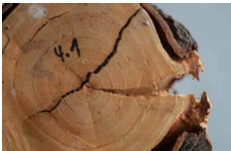
Hawthorn stem ( Crataegus laevigata ) after mechanical load test. Increasing compressive loading until fracture of the wood resulted in data for the „Stuttgarter Festigkeitskatalog (Stuttgart Strength Catalog)“ (joint project of Technical Biology [U. Kull] and Engineering [Structural and Model Statics] of the University of Stuttgart; 1995). (Botanical Collection)
